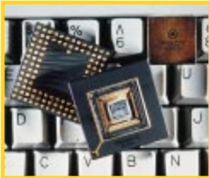
**1984** Motorola introduces the MC68020 with 250,000 transistors.
