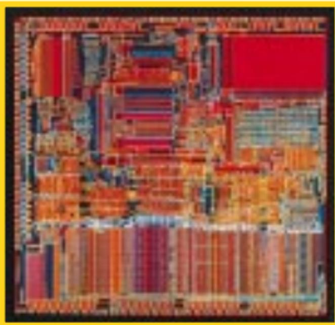
**1985** In October, Intel introduces the 80386 chip with 32-bit processing and on-chip memory management.
