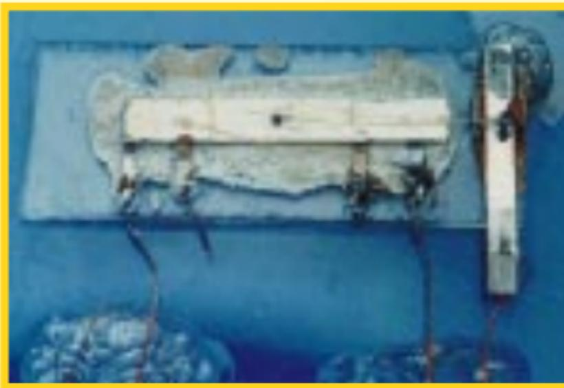
**1958** At Texas Instruments, Jack Kilby develops a prototype semiconductor IC while Robert Noyce works separately on ICs at Fairchild Semiconductor.
