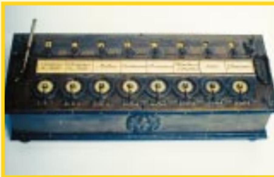
**1642-1643** Blaise Pascal creates a gear-driven adding machine called the "Pascalene," the first mechanical adding machine.
