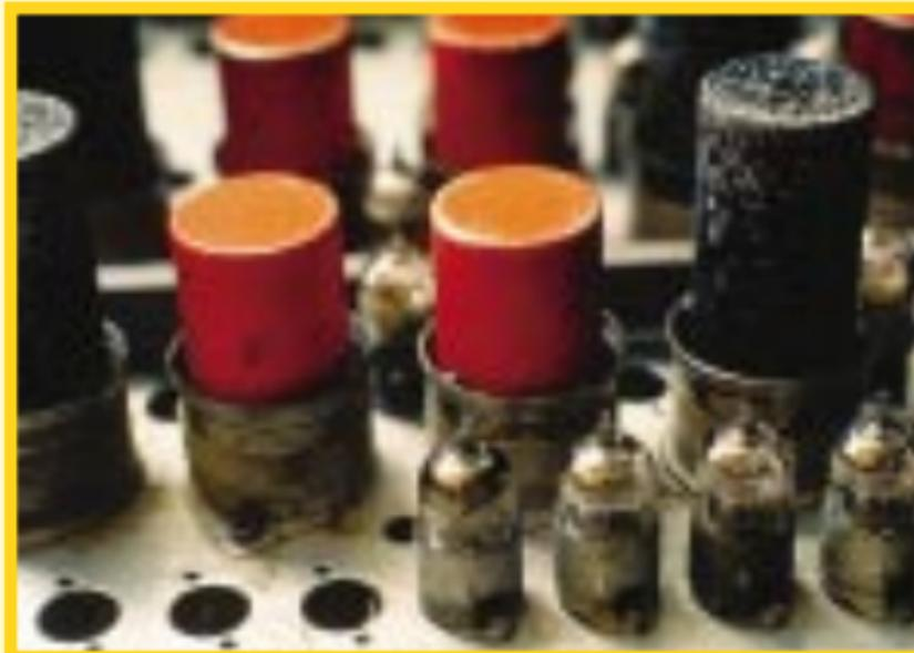
**1948** On June 21, the Manchester Mark I, or "baby" machine, becomes the first operational stored-program digital computer. It used vacuum tube, or valve, circuits.
